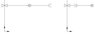
In both cases, the end-effector cannot move instantaneously in the  $\hat{X}_0$  direction, i.e. the joints cannot produce a velocity component in the  $\hat{X}_0$  direction.
