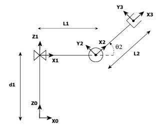
(a) Find the origin of frame  $\{3\}$  expressed in terms of frame  $\{0\}$ , that is  ${}^{0}\mathbf{P}_{3org}$ . Tip: you can derive this geometrically, if you want to avoid going through DH parameters. It's simplest to do this geometrically. Note: I will often refer to the origin of frame  $\{3\}$  as the "tip".
