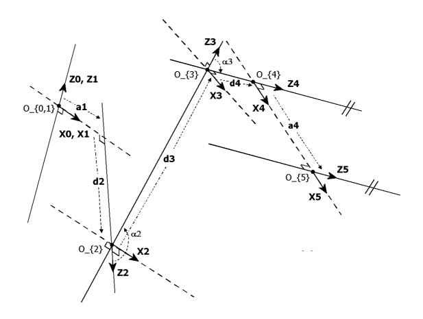
$(b) \ \mbox{Write down the Denavit-Hartenberg parameters for this manipulator, in the form of a table:$
