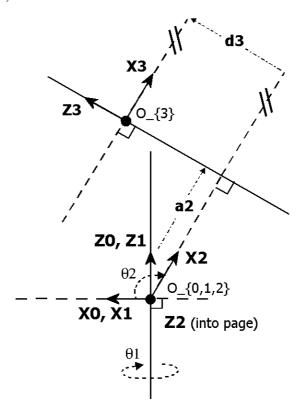
(b) Write down the Denavit-Hartenberg parameters for this manipulator, in the form of a table:
