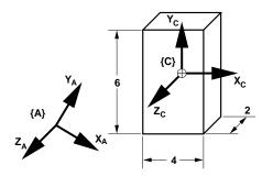
Frame  $\{C\}$  lies at the center of mass of the box, and the coordinate axes are ligned up with the principal axes of the box. In other words,  $\mathbf{Y}_C$  is aligned with the long axis of the box, and  $\mathbf{X}_C$  and  $\mathbf{Z}_C$  are aligned with the short axes of the box.
