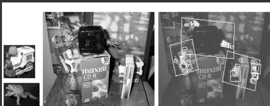
Figure 12: The training images for two objects are shown on the left. These can be recognized in a cluttered image with extensive occlusion, shown in the middle. The results of recognition are shown on the right overlaid on a reduced contrast version of the image. A parallelogram is drawn around each recognized object showing the boundaries of the original training image under the affine transformation solved for during recognition. Smaller squares indicate the keypoints that were used for recognition.
